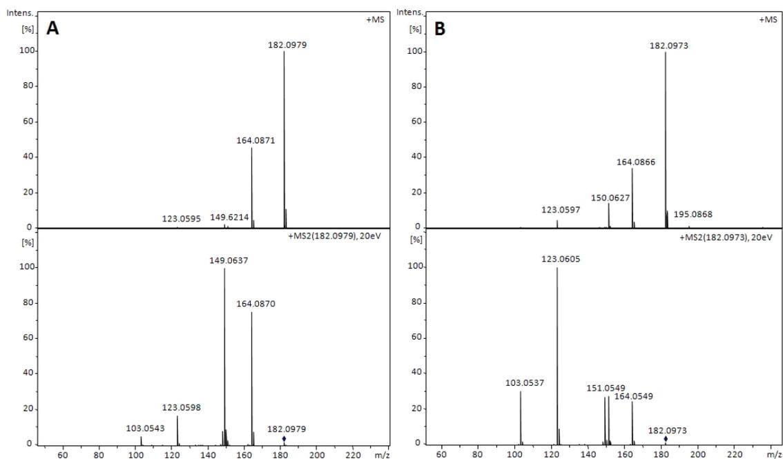
**Figure 4:** MS and MS/MS (+MS2) spectra obtained for 3-FMC (A) and 3-isoFMC (B).
