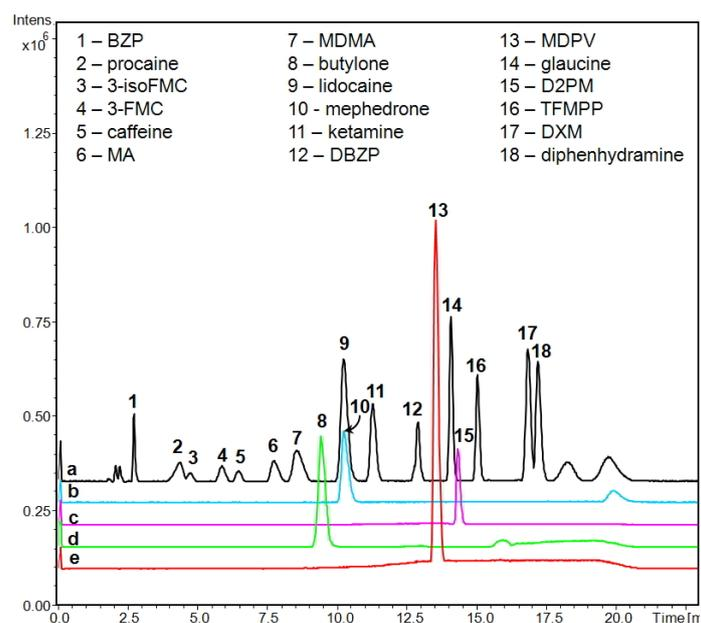
**Figure 3:** Total Ion Chromatograms (TIC) recorded for the mixture of 13 compounds (a), mephedrone solution (b), D2PM solution (c), butylone solution (d), MDPV solution (e).
