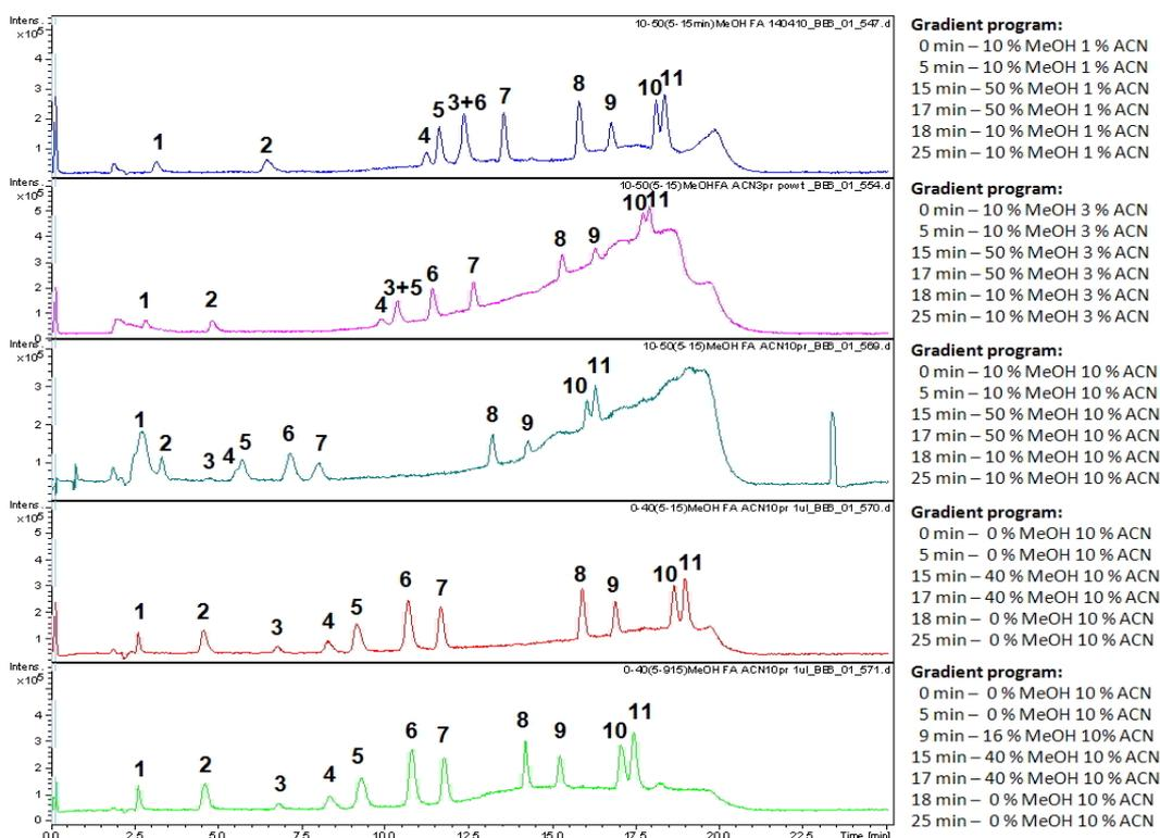
**Figure 2:** Total Ion Chromatograms (TIC) recorded for different gradient programs with ACN/MeOH mixture as an organic modifier of the mobile phase; Identified peaks: 1 – BZP, 2 – procaine, 3 – caffeine, 4 – MA, 5 – MDMA, 6 – lidocaine, 7 – ketamine, 8 – glaucine, 9 – TFMPP, 10 – DXM, 11 – diphenhydramine
