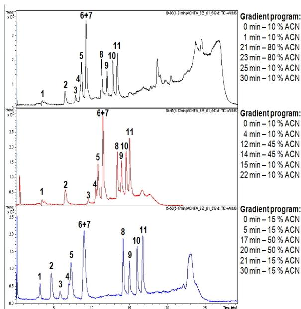
**Figure 1:** Total Ion Chromatograms (TIC) recorded for different gradient programs with ACN as an organic modifier of the mobile phase; Identified peaks: 1 – BZP, 2 – procaine, 3 – caffeine, 4 – MA, 5 – MDMA, 6 – lidocaine, 7 – ketamine, 8 – glaucine, 9 – TFMP, 10 – DXM, 11 – diphenhydramine.
