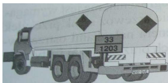
**Figure 3:** Example of correctly labelled tanker carrying only one dangerous substance.
