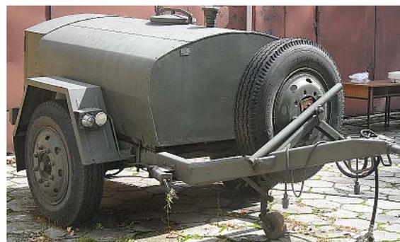
**Figure 2:** Water wagon with a capacity of 1,000 dm<sup>3</sup>.
