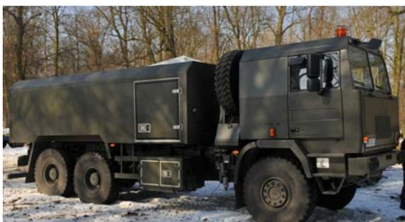
**Figure 4:** Water tank for transporting up to 10 m<sup>3</sup> of water.
