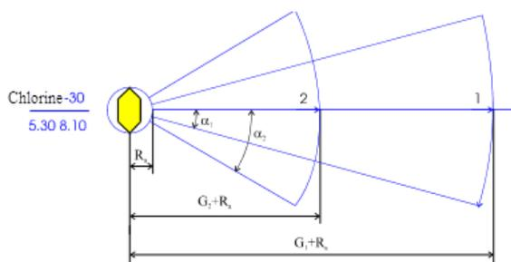
**Figure 1:** A diagram of expected contamination zones after the accident of a plant using toxic industrial materials.
